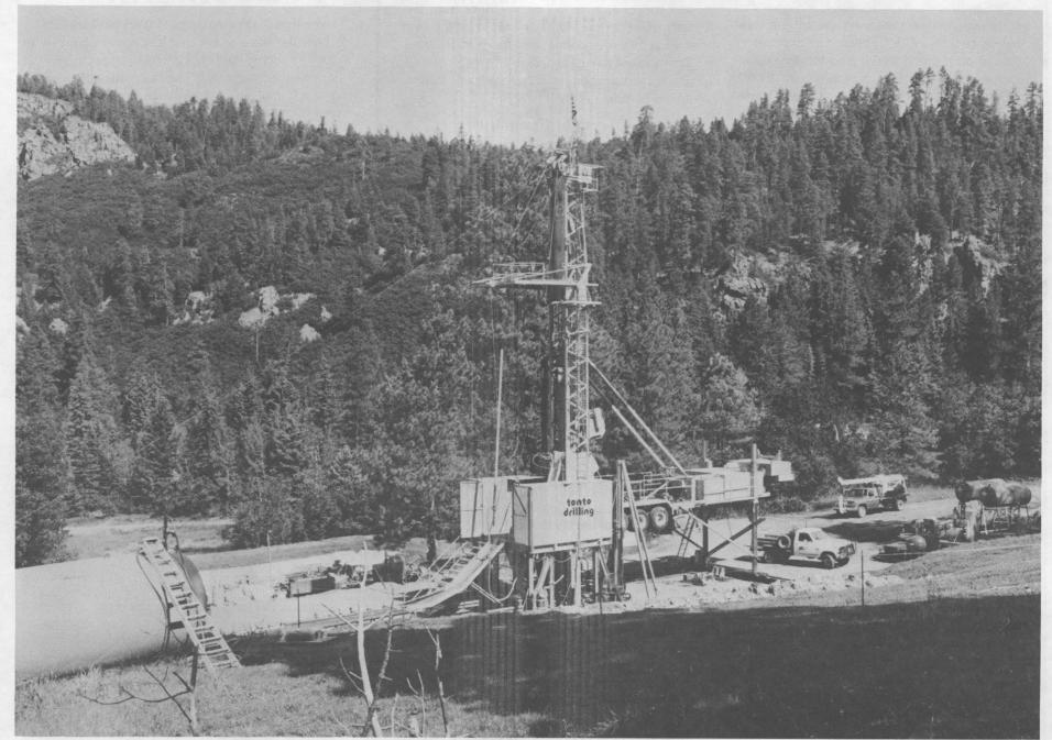
VALLES CALDERA COREHOLE drilling, completed last month, was both a scientific and an engineering success. The corehole, part of the Continental Scientific Drilling Program, reached a depth of 5780 feet and a high-temperature (>570°F) geothermal zone. Site is on private land in the Jemez Mountains north of Albuquerque.
